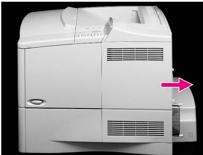
Figure 40. Removing the rear right side cover
