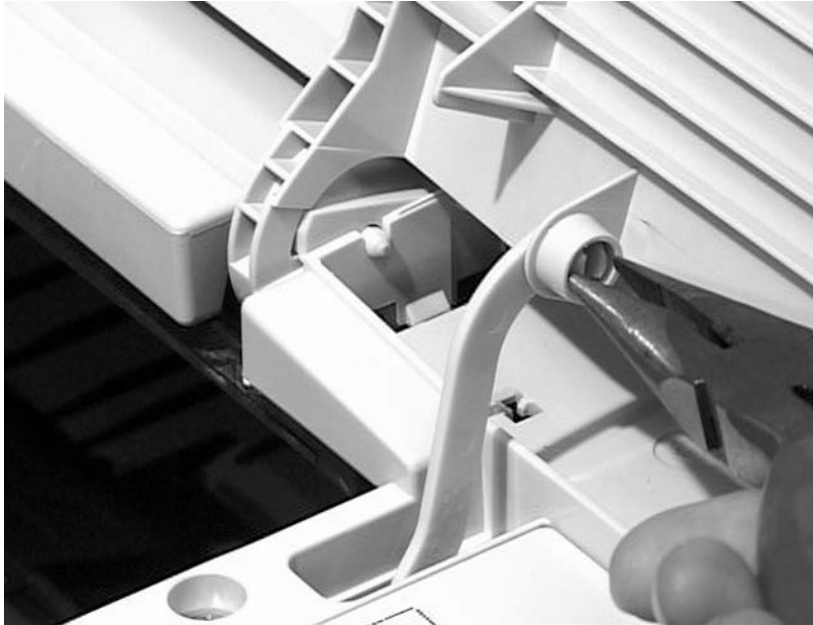
Figure 43. Disconnecting the toner cartridge drive arm
